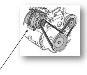
The pulley on the end of the crank shaft drives a fan pulley and an "Alternator" pulley. The **tension** is achieved by moving the alternator away from the engine pulling the belt tight. The alternator is then locked in position by means of a locking bolt.
